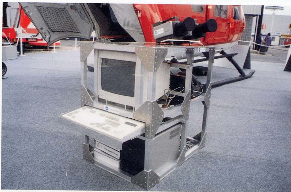
Fig. 3.3: The AGEMA measurement equipment with the 3-5 \mu\text{m} and the 8-12 \mu\text{m} scanner mounted in an Aluminium-Rack is ready for helicopter flight trials.
