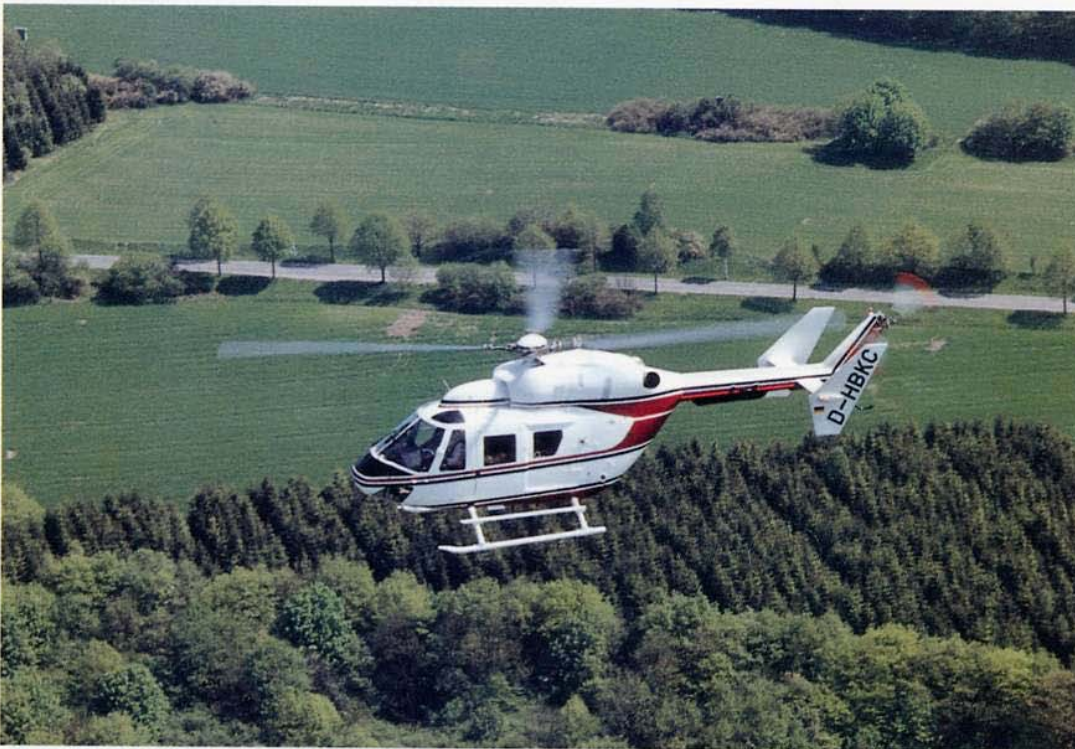
Fig. 3.1: The BK117 helicopter from EUROCOPTER with a max. take-off weight of 3.350 kg in a hilly landscape
