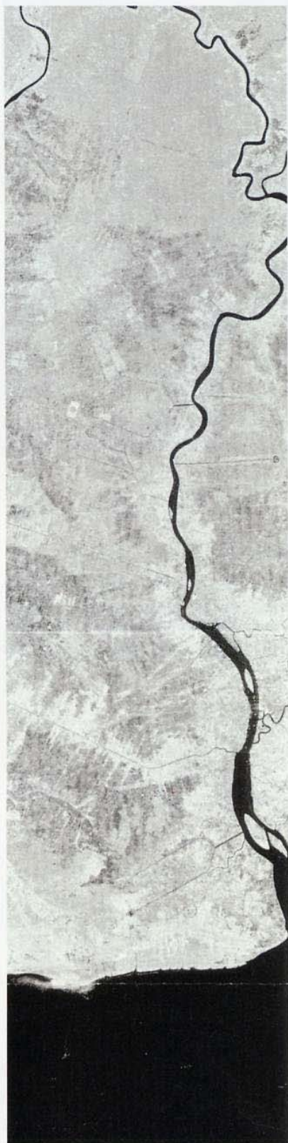
Fig. 5.3: A section of ERS-1 image from 6. 5. 1993 showing the mountains area in Kalimantan Tengah in the eastern part of Schwaner Mountain (approx. 40 km x 70 km); processed by W. Bergbauer (Red = 15x15 convolution matrix, green = \sigma 7 speckle filter, blue = 31x31 convolution matrix)
