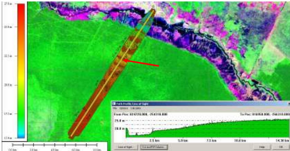
**Figure 9.** LiDAR-DTM of CIMTROP transect in Sabangau National Park with 1m contour-lines and peat topography profile, Landsat image from 5.8.2007. The red arrow shows the highest slope of the transect with 0.17%.
