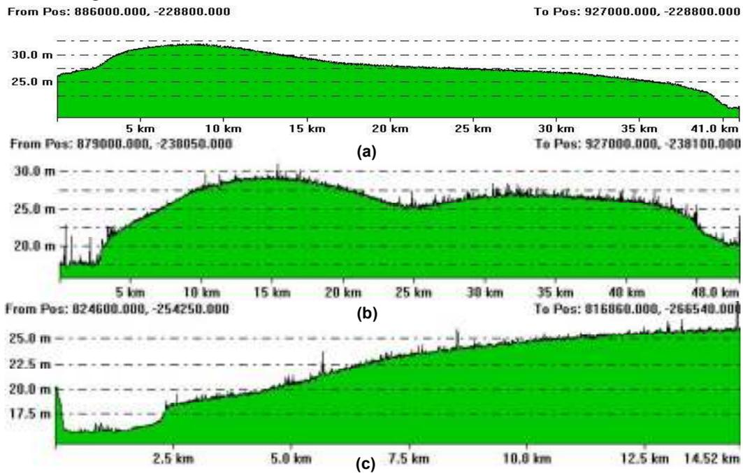
**Figure 2.** LiDAR-DTM profiles for Mawas area in (a) km228.8 and (b) km238 and (c) Sabangau area. We selected for the cross-section a profile parallel to the visible logging transects. Transects were acquired with different lengths and have different scales.
