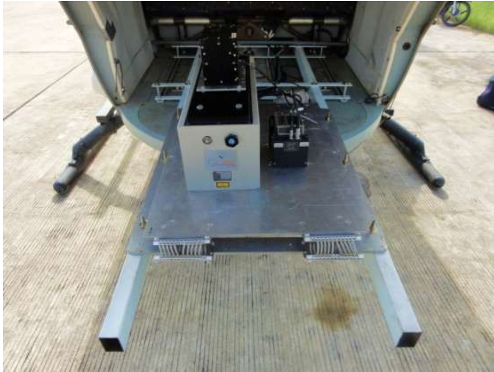
BK117 Avionic Bay with LiDAR – and Hasselblad-equipment
